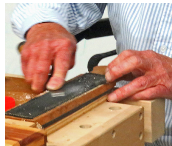
Stropping with Yellowstone Compound
